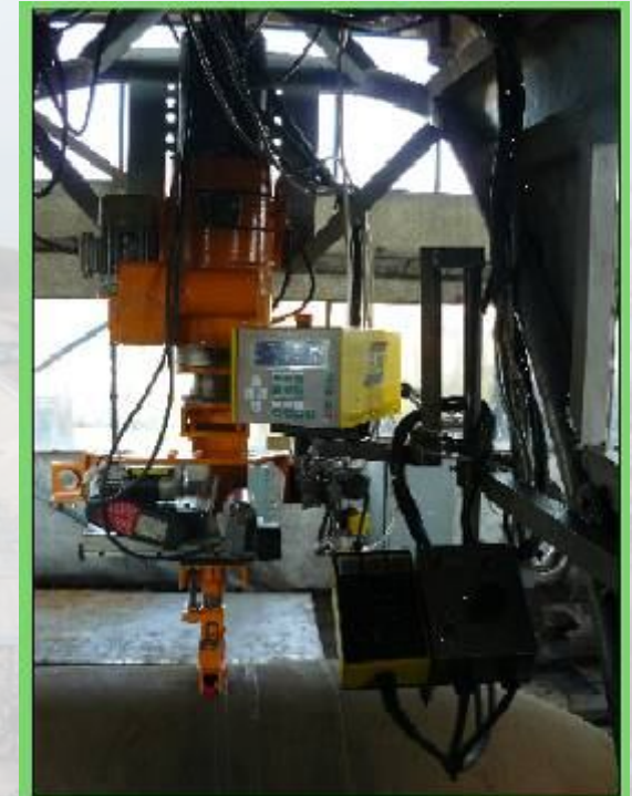
Welding head with control panels (automatic welding operator's work station)
